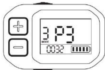
P3: setting the speed limit within 0-25km/h; The default speed limit is 25km/h.
