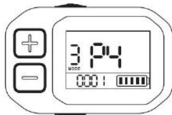
P4: setting the default speed level; 0 means starting at speed level 0, and 1 means starting at speed level 1.
