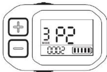
P2: setting the screen timeout within 0-30 minutes; 0 means it never sleeps.
