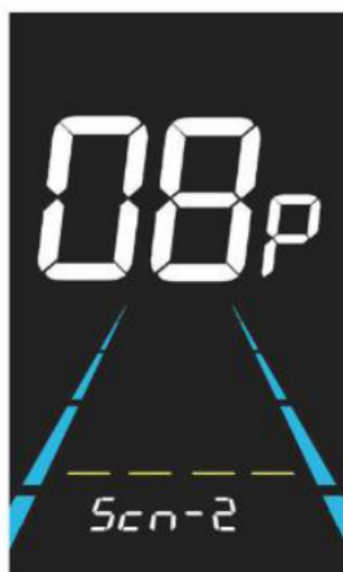
Figure 6-10 PAS sensor sensitivity setting interface
