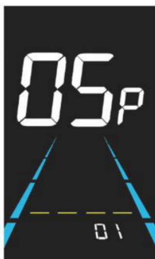
Figure 6-6 Number of speed sensor magnets setting interface
