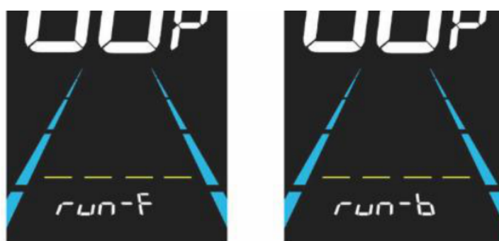
Figure 6-9 PAS sensor direction setting interface
