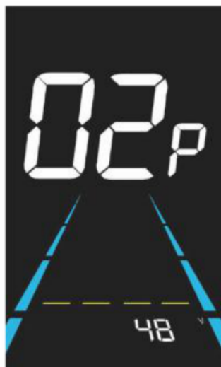
Figure 6-2 Rated voltage setting interface
