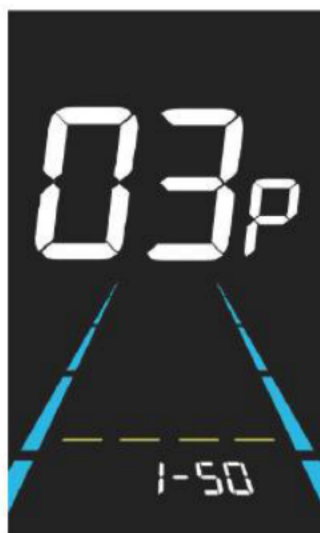
Figure 6-4 PAS level ratio value setting interface
