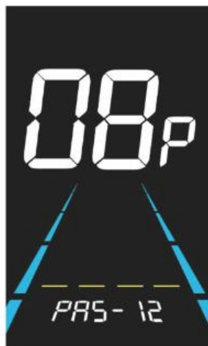
Figure 6-11 Pedal assist sensor magnets setting
