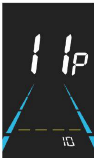
Figure 6-17 Auto Power Off Time Setting Interface
