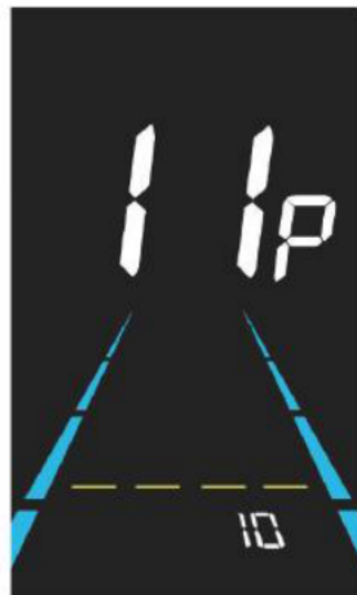
Figure 6-17 Auto Power Off Time Setting Interface
