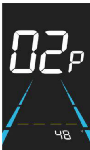
Figure 6-2 Rated voltage setting interface
