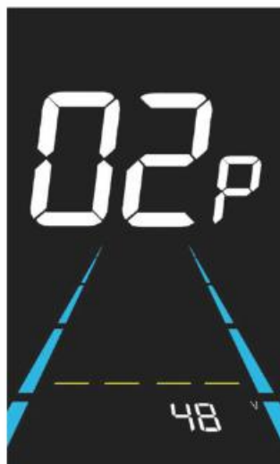
Figure 6-2 Rated voltage setting interface
