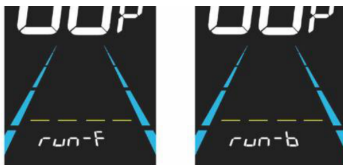
Figure 6-9 PAS sensor direction setting interface
