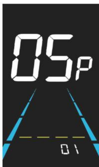
Figure 6-6 Number of speed sensor magnets setting interface
