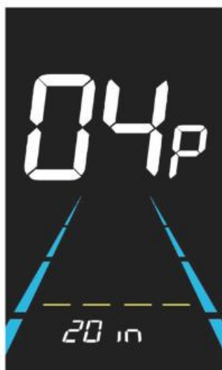
Figure 6-5 Wheel diameter setting interface
