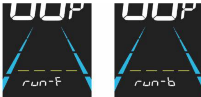
Figure 6-9 PAS sensor direction setting interface
