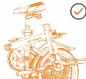
4 Open the frame latch and adjust the left pedal (without interfering with folding)
