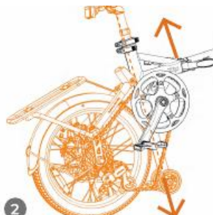
2 Hold the top tube and push the saddle fully down
